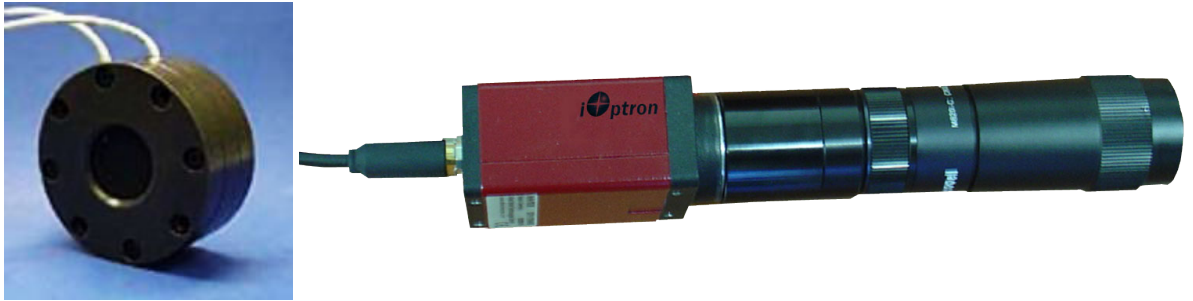
Left: Hyperspectral filter. Right: Camera with BATi's tunable filter.
