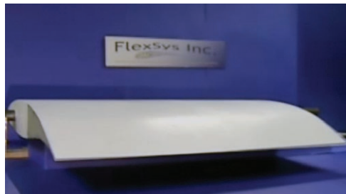
FlexSys' mission adaptive compliant trailing edge was designed for a high-altitude, long-endurance aircraft undergoing 10^9 flap deflection with a 3^\circ twist.
