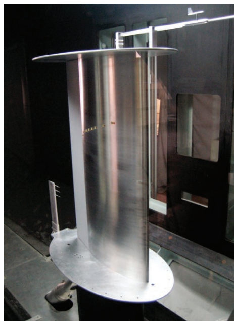
A laminar-flow flight test model fitted with variable geometry trailing edge.
