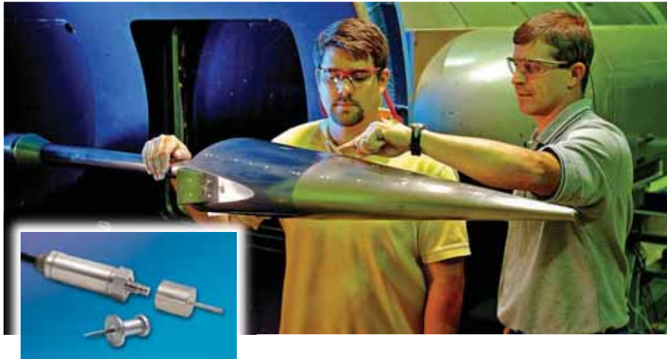
Successful demonstration of the manufactured 5 psi transducer was performed at AEDC in both Precision Measurement Equipment Lab and in Hypersonic Wind Tunnels B & C.
